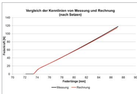
The simulation model developed by the SCHERDELGroup lies on the calculated curve with an error of less than five per cent.
